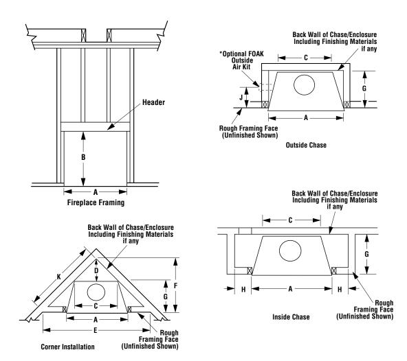
**Note:** All framing dimensions calculated for 1/2" dry wall at the appliance face. If sheathing the chase or finishing with other thickness materials, calculations will need to be made.
